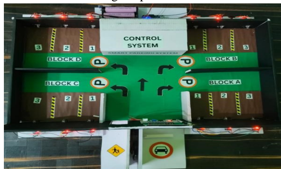
Fig. 2 Block-wise representation of Smart Parking System
