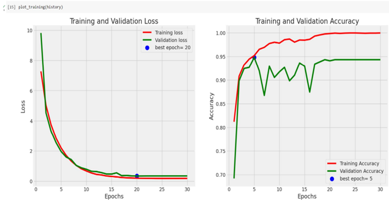
Figure.12. Training and validation Loss, accuracy Plot
