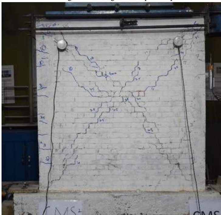
Figure 7: Damage pattern before retrofitting
