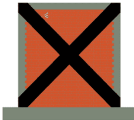
Figure 6. FRP Retrofitting configuration
