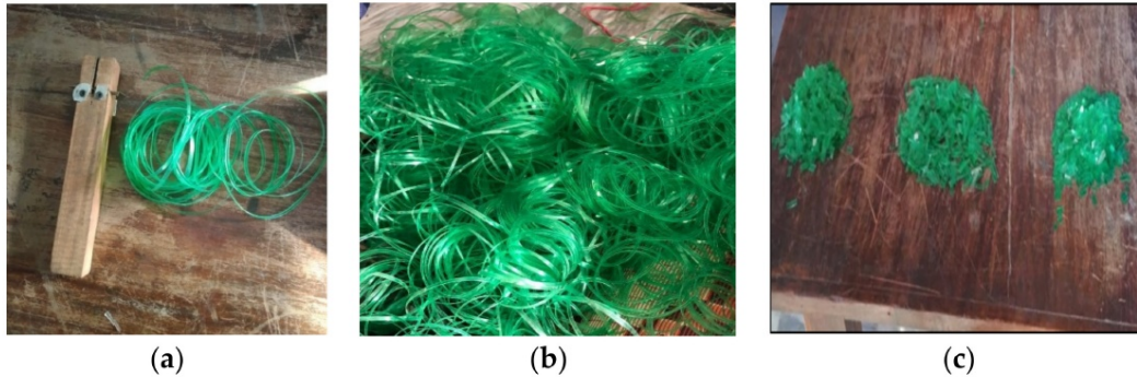
Figure 1. Waste PET bottle strip process: (a) strip cutting tool; (b) PET spiral; (c) plastic strips sizes.
