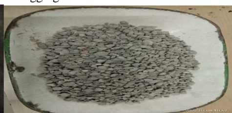
Fig 2: Heated & abrasioned aggregates
