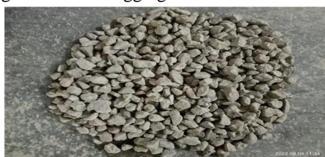
Fig 3. Heated abrasioned & Silica Fume treated aggregates
