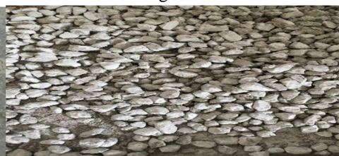
Fig 4. Heated abrasioned & Fly ash treated aggregates
