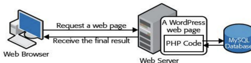
Fig. 2 Working relation of client ,server and database in web CMS [8]
