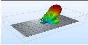
each element produces an equal output voltage of  $sin(\omega t)sin(\omega t)$ . However, there will be an equal phase difference  $\Psi\Psi$  between successive elements. Mathematically, it can be written as  $-\Psi=2\pi dsin\theta\lambda Equation1\Psi=2\pi dsin\theta\lambda Equation1$  Where,  $\theta$  is the angle at which the incoming signal isincident on each radiation element.
