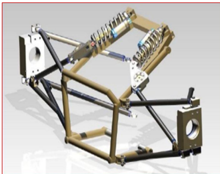
Fig.1.2. Rear Suspension Assembly
