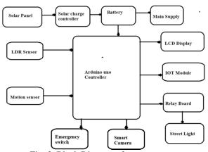
Fig. 3. Block Diagram of system
