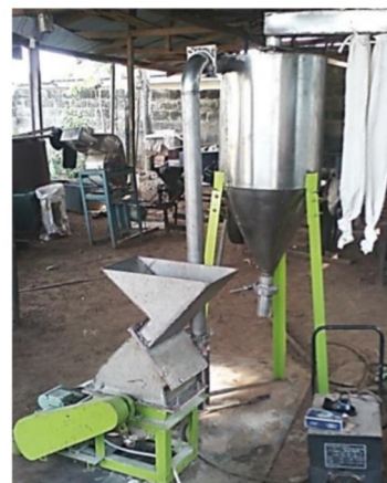
Fig. 12. The fabricated pulverizer
