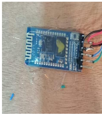
Fig 6: HC-05 Bluetooth module setup
