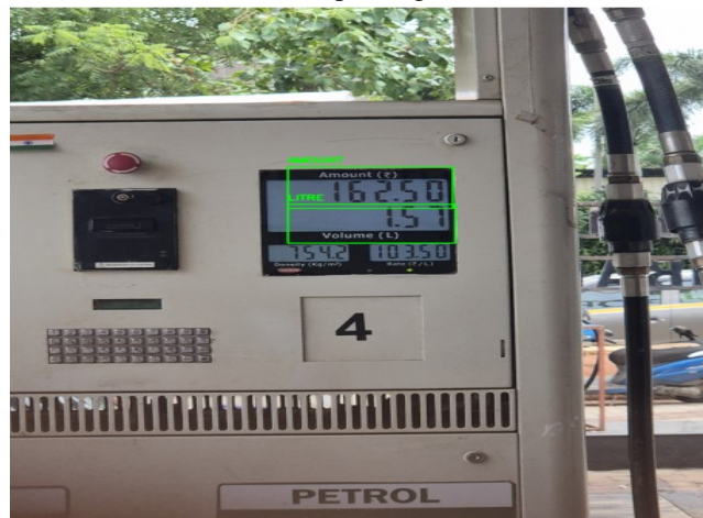
Fig. 1. Example of ROI detection using YOLOv8 on a fuel pump display
