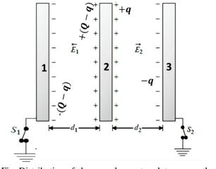
Fig. Distribution of charges when outer plates are earthconnected
