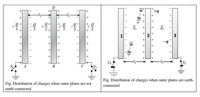
Now, the electric field intensity between plate 1 and 2 is  $E_1 = \frac{Q-q}{\epsilon_0 A}$ The electric field intensity between plates 2 and 3 is  $E_2 = \frac{q}{\epsilon_0 A}$ Now, using Kirchhoff's voltage law, we can write
