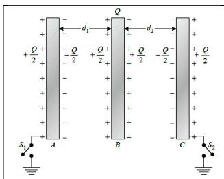
Fig. Distribution of charges when outer plates are not earth-connected
