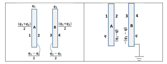
Now, we consider the case when one of the plates is earth-connected, and due to the earth connection, the distribution of charges will be different. Let due to the earth connection, the charge appears on the outer surface of plate 1 and 4 is q. So, the Charge on the inner surface of plate 1 is  $(q_1 - q)$ , and the inner surface of plate 2 is  $\{-(q_1 - q)\}$ .
