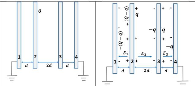
From the above discussions, we learned that the charge on the outer surface of earth connected plate is zero, so charge on the outer surface of plate 1 & 4 have no charge.
