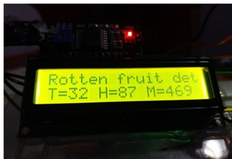
Fig 7: LCD display displaying sensors values
