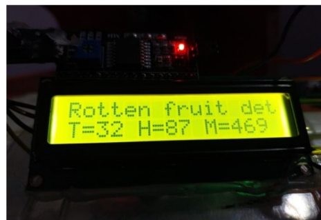
Fig 7: LCD display displaying sensors values
