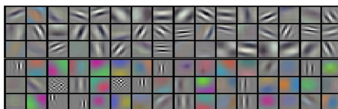
Fig. 2. Examples of the image feature detectors that a CNN might “learn” during its training [6].
