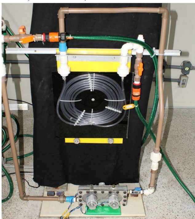
Fig. 8 Ultrasonic reactor assembled in the calcium carbonate scaling plant.
