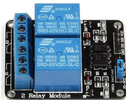
FIG: 3 2 CHANNEL RELAY
