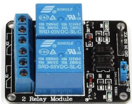
FIG: 3 2 CHANNEL RELAY
