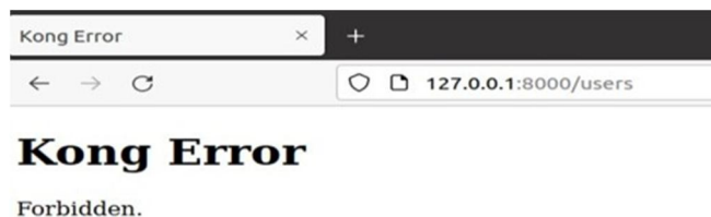
Fig. 4. Getting Forbidden message as a response from the /users endpoint. And for the next test case we have restricted our system IP address using the IP restriction plugin.
