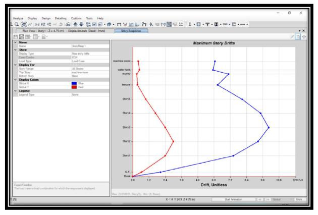
Max Storey Drift For Y Direction In Shear Wall
