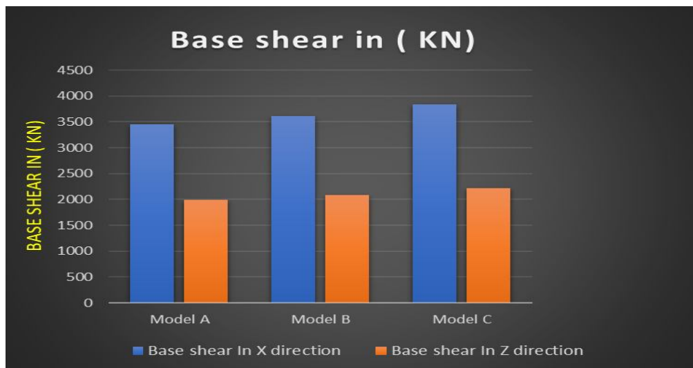
Fig. 14: Base shear values due to the Response spectrum method in X and Z direction for all Models.
