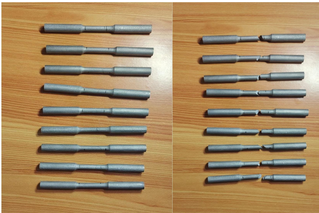
Figure 5: UTM L9 samples and after experimental braked samples.
