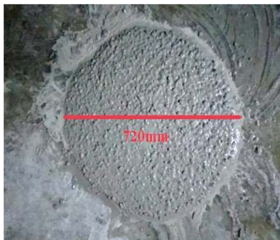
Fig. 4.8 Slump Flow of trial mix number - TM16
