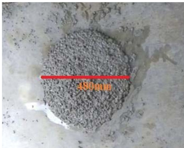
Fig. 4.7 Slump Flow of trial mix number - TM25
