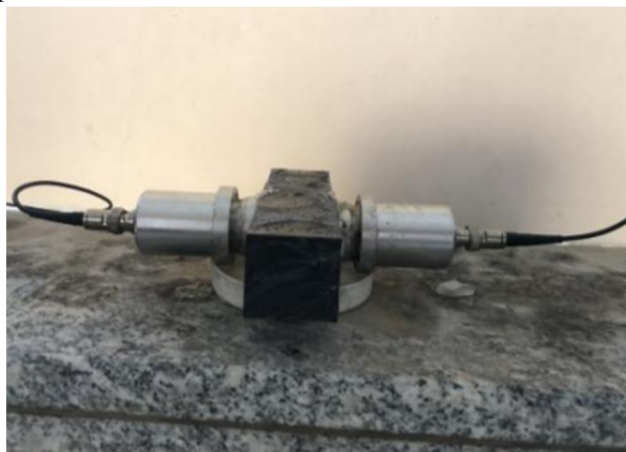
Fig 7 Set up of UPV test. [23]
