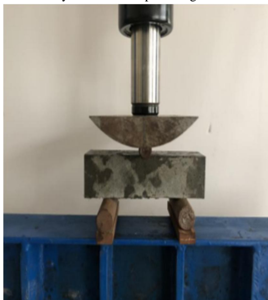
Fig 5. 3-Point Bending Test Setup [23]
