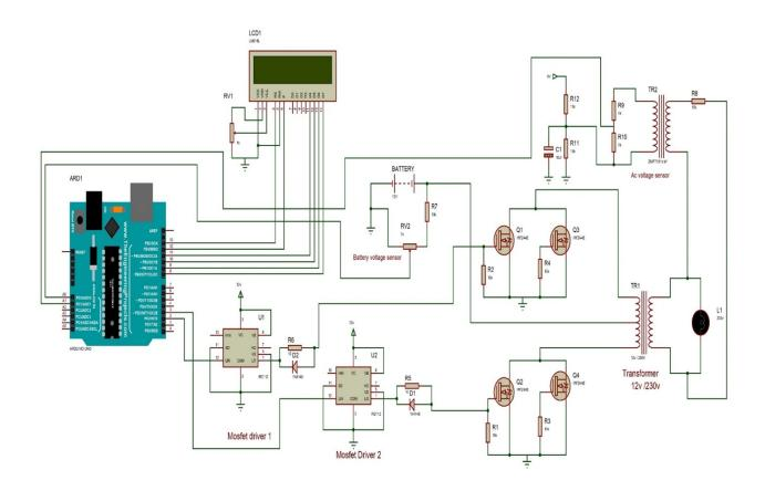
Circuit Diagram Of Single Phase Inverter Using Pwm Technique
