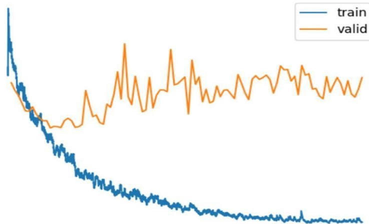
Fig 1 :Loss Plot Graph showing overfitting of the model (ResNet50)
