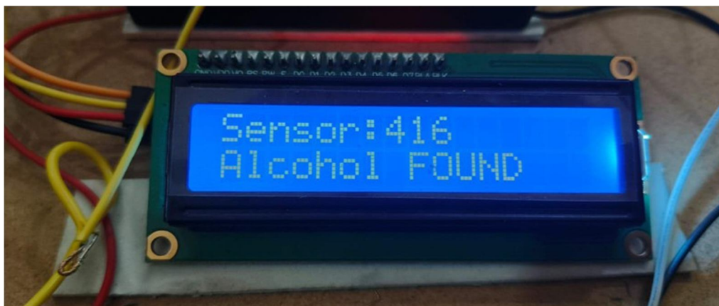
Fig.5 Showing alcohol found on lcd screen
