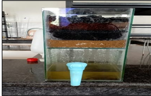
Figure 4.6 Filtration Media and its process
