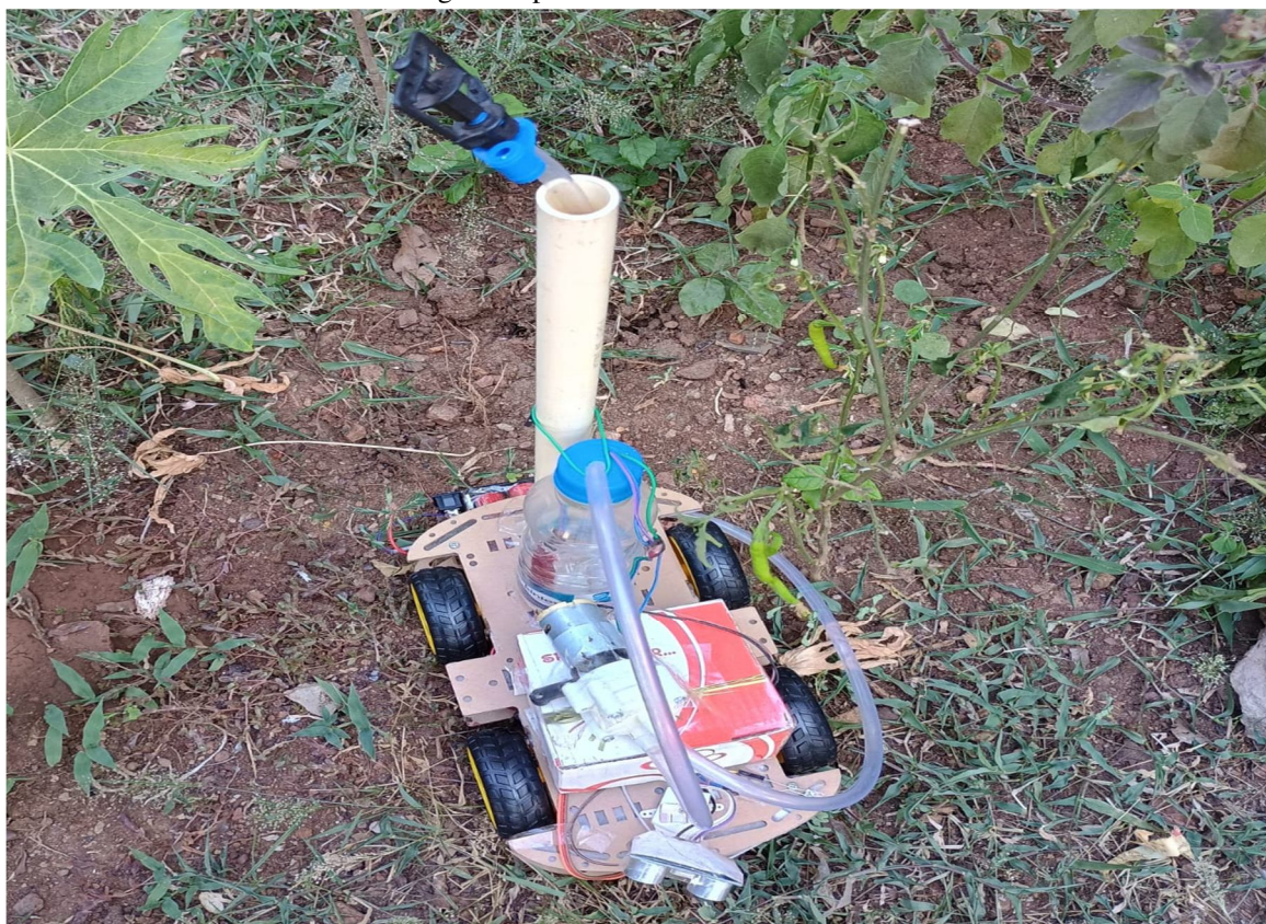
Fig. 2 Smart Automatic Liquid Sprinkler Robot
