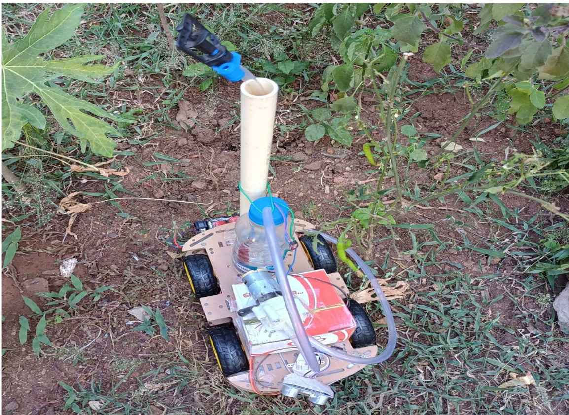
Fig. 2 Smart Automatic Liquid Sprinkler Robot
