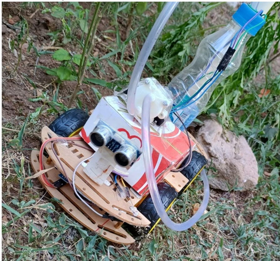
Fig. 5 Robot front view displaying servo motor and ultrasonic sensor
