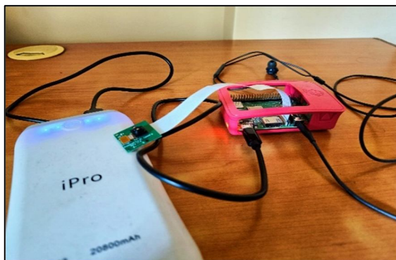
Fig 12: RPI Camera Connected with Raspberry Pi 3B+
