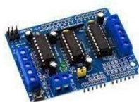
Fig.2.7- A L293D Motor driver
