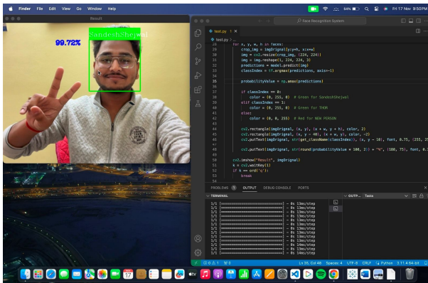
Fig 4.1 Screenshot of Face Recognition output where name of trusted person and the accuracy is mentioned.
