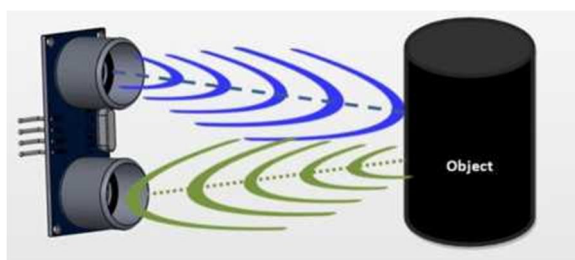
Fig. 3: Working of Ultrasonic Sensor
