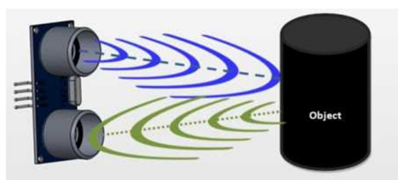
Fig. 3: Working of Ultrasonic Sensor
