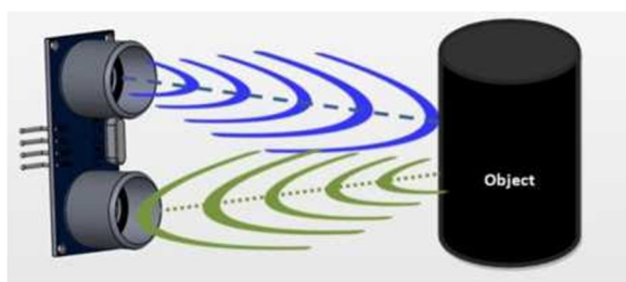
Fig. 3: Working of Ultrasonic Sensor
