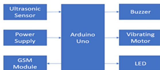
Fig. 3: Block diagram of Smart Guidance Belt
