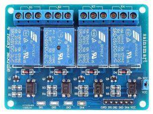
In this setup, the relay module is interfaced with the GPIO pins of the ESP32 microcontroller, which sends the necessary control signal to activate or deactivate the relay. This allows for the switching of connected appliances or devices, such as light bulbs, based on real-time inputs or pre-configured scenarios.
