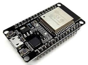
In this project, the ESP32 serves as the central processing unit (CPU), responsible for managing all control logic and communications. The user-written program is uploaded to the ESP32, which interacts with peripheral devices such as relays and sensors through its GPIO pins. The relays are used to control household appliances, while sensor data inputs are processed to enable real-time decision-making and cloud synchronization, as depicted in Fig. 2.
