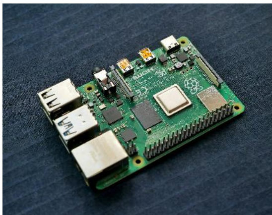
Figure 2: Raspberry Pi 4 onboard controller
