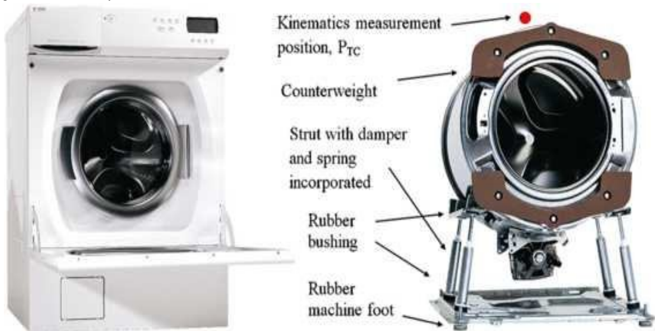
Fig. 4: Application of Magneto-Rheological Fluids in Household Appliance
