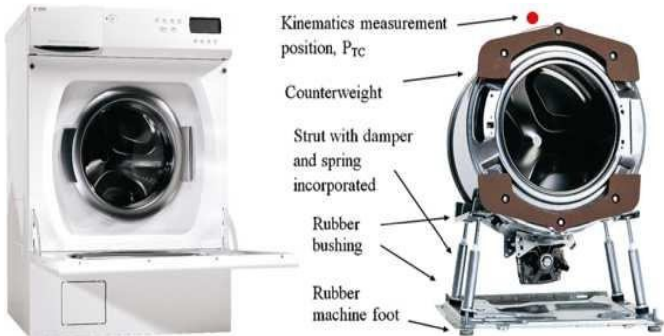
Fig. 4: Application of Magneto-Rheological Fluids in Household Appliance
