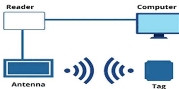
Fig(1) :- Working of RFID System with
