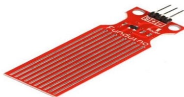
Figure-3. Water level Sensor.
