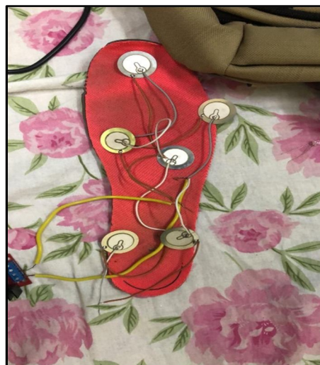
Fig. Piezoelectric chips on Shoe sole
