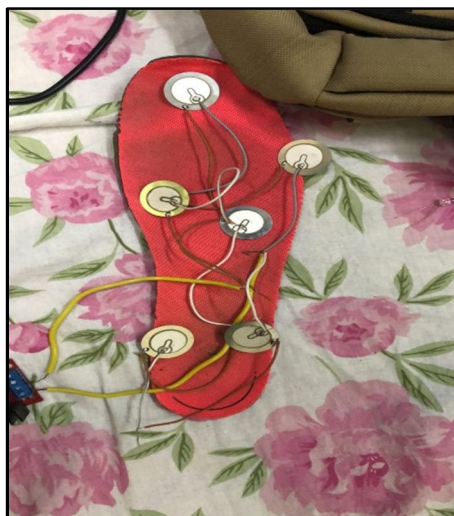
Fig. Piezoelectric chips on Shoe sole
