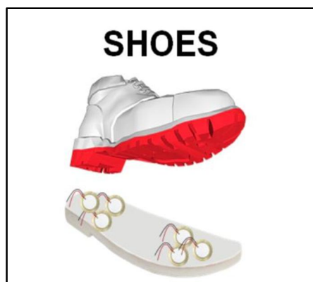
Fig. Piezoelectric chips on Shoe sole
