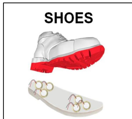
Fig. Piezoelectric chips on Shoe sole
