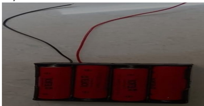
FIG NO7.3.1:- LI-ION Battery Set
