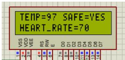
Fig -5: Output from the proteus simulation
