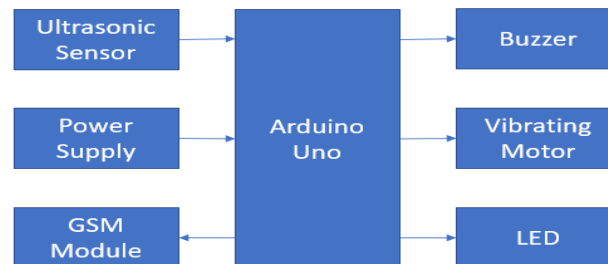
Figure 5: Block Diagram of Smart Wearable Guiding Device
