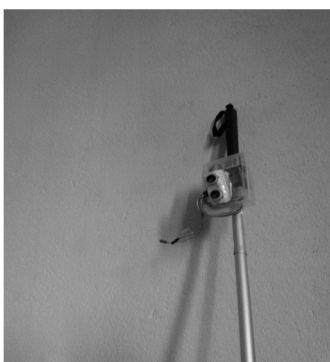
Fig.7: Prototype 2: Using Vibration motor
