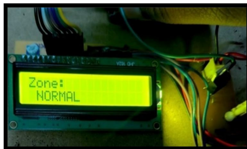
Fig. 6 Image of the LCD display for NORMAL ZONE
