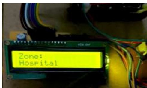
Fig. 8 Image of the LCD display for HOSPITAL ZONE
