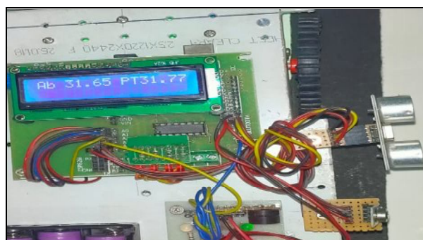
Fig.6 Contactless Temperature measurement is done by MLX90614 sensor.
