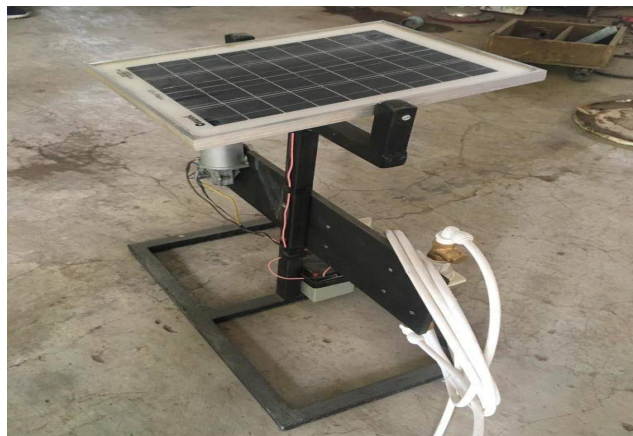
Fig. 1: Solar power reciprocating pump
