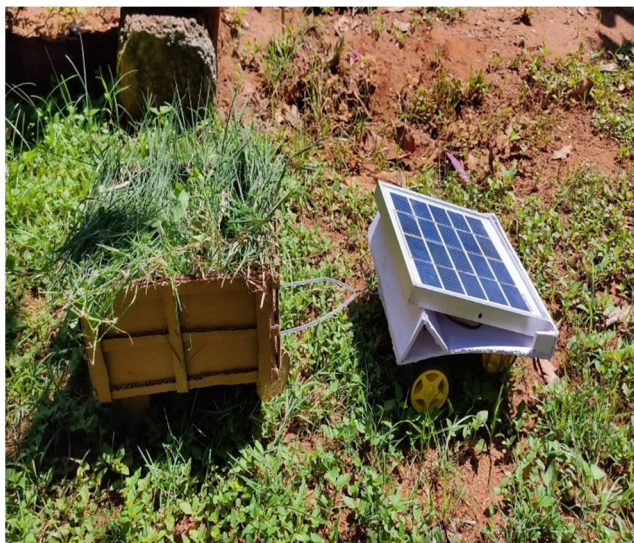
Figure 3: Solar Driven Agri Bot for transporting loads in agriculture land
