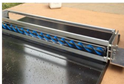
The Selected Brush Design Installed on Prototype
