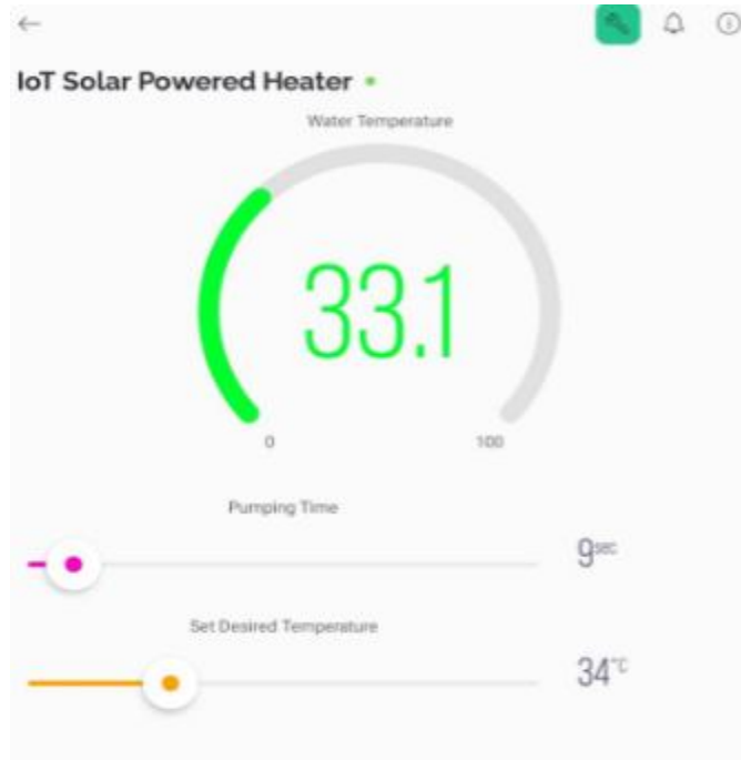
Fig.4. Controlling of the system (pumping time and set desired temperature) through Blynk app
