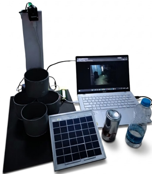
Fig.4.Experimental Setup of Solar-Based E-Waste Sorting Robot
